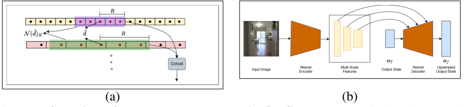
Figure 2: Overview of the proposed modules in OptSplat. (a) Iterative local cost volume extraction: At each refinement step, we dynamically index a global cost volume using the current depth estimate to construct localized cost volumes for recurrent depth refinement. (b) Appearance-Guided Upsampler: A UNet-style architecture upsamples the final hidden state o^T to the input image resolution, producing dense 3D Gaussian parameters guided by image appearance features.
